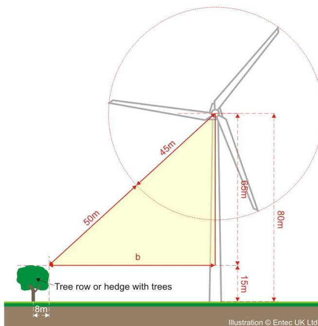
where: bl = blade length, hh = hub height, fh = feature height (all in metres). For the example above, b = 69.3 m.
